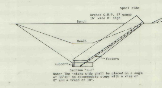
NOTE: The maximum slope of any spoil bank shall be limited to 30 degrees.
