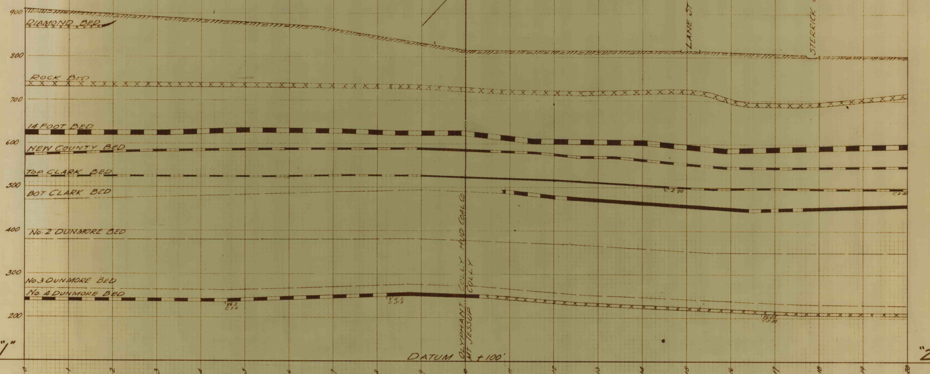
CROSS SECTION OF THE SEVERAL BEDS THRU OLYPHANT & MT. JESSUP COLLIERIES. ~ AT RIGHT ANGLES TO COMMON BOUNDARY LINE 1640' FROM S.E. CORNER OF PROPERTY (S.S. #82) OFFICE OF THE MINING ENGINEER, HUDSON COAL CO. SCRANTON PA. SCALE 1"=100' OCT. 12, 1931.
