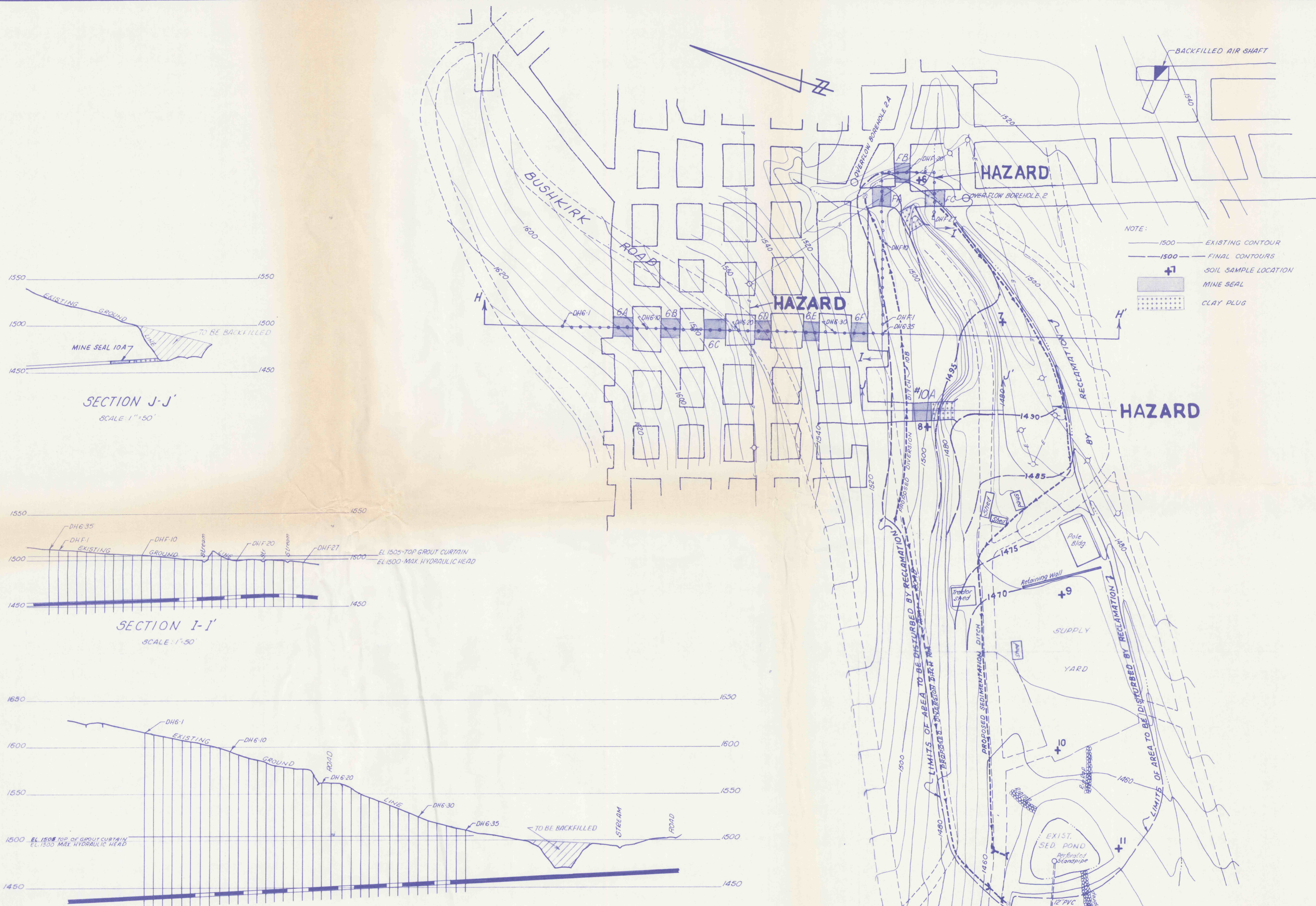
PLAN OF MINE SEALS NO 6, 10, FAN & OVERFLOW BOREHOLE 2 DEEP MINE HYDRAULIC SEALS & PRESSURE GROUTING DRILL HOLES SCALE: 1" = 50'
