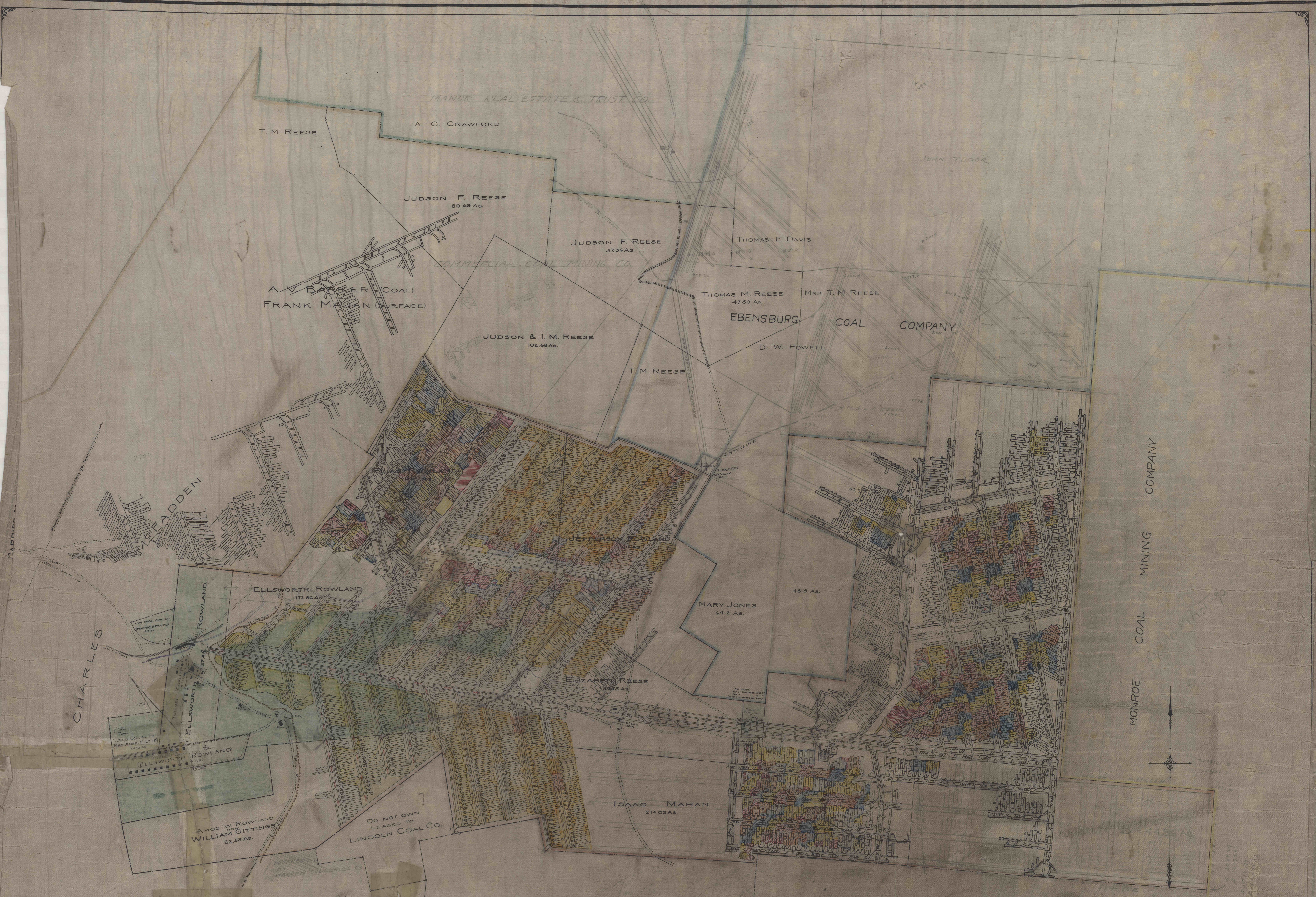
MAP OF CARDIFF COAL CO'S MINE SITUATE NEAR NANTY-GLO ON BLACK LICK BRANCH OF CRESSON DIV. P.R.R. BLACK LICK TWP., CAMBRIA CO., PA. SCALE: 1 IN. = 400 FT. MINE WORKINGS SHOWN AS PER SURVEY OF ENGINEER
