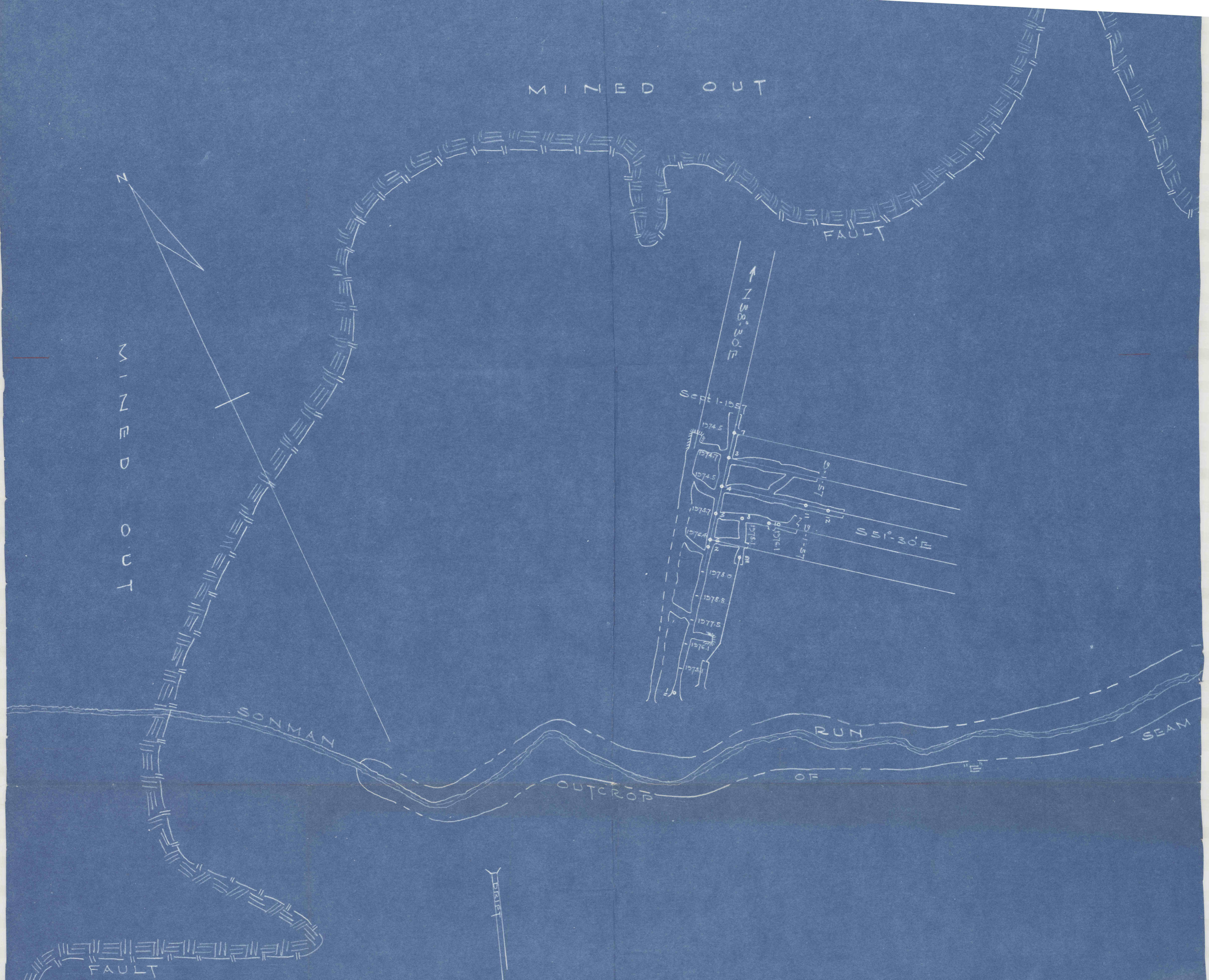
MAP SHOWING MINE WORKINGS OF PROSITY COAL CO. ON "E" SEAM LANDS OF CAMBRIA MINING & MFG. CO. NEAR SHOEMAKER-CAMBRIA CO.-PA. SCALE 1"=100' SEPT-1957
