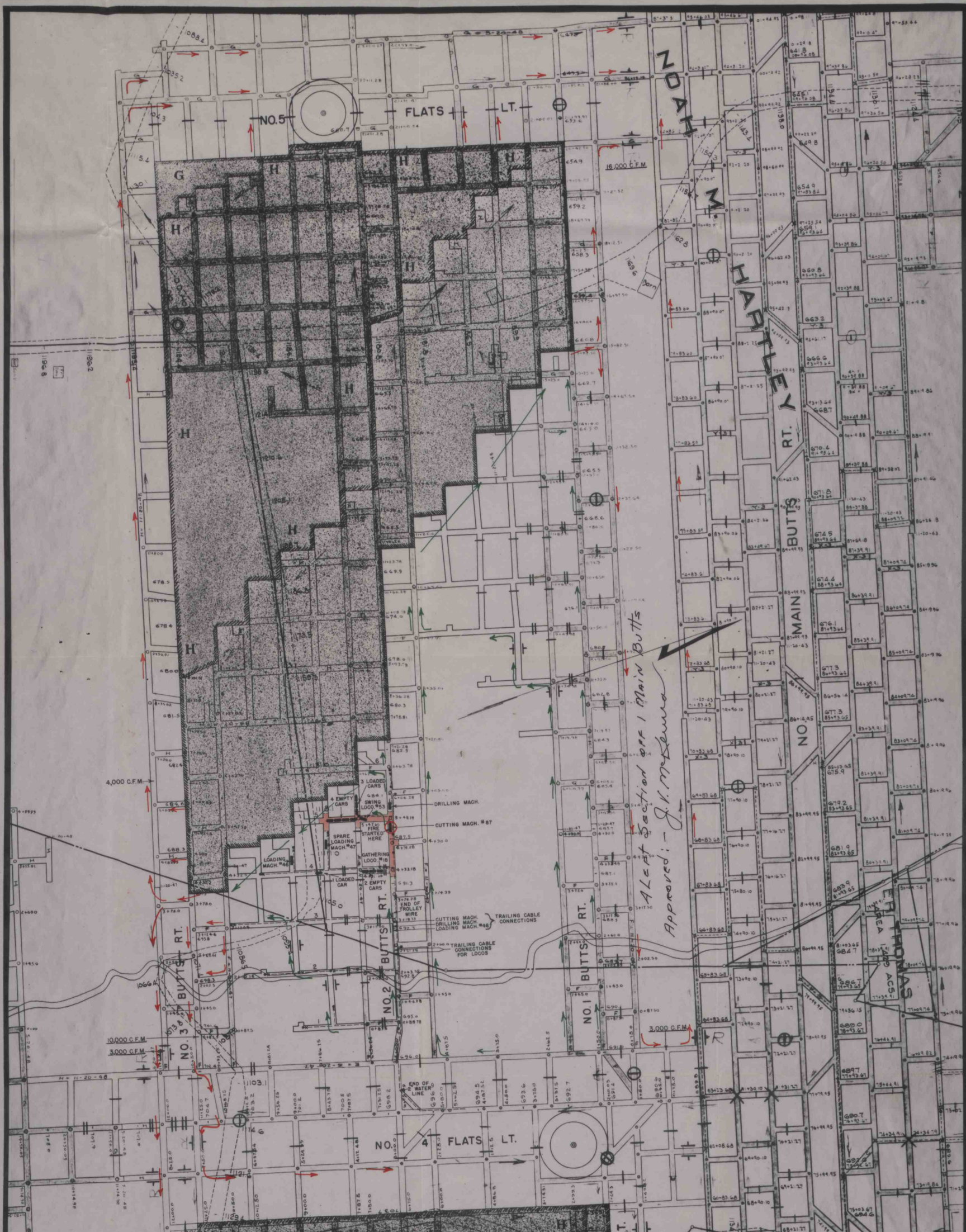
ROBENA MINE Map Showing Fire Area, Position of Equipment, and Ventilation just prior to start of Fire on Feb. 11, 1949 Scale 100' 0' 100' 200' Feb. 22, 1949 LEGEND Maximum extent of Fire Stoppings with Doors Intake Air Doors Return Air Regulators Overcast Water Valves Stoppings Water Taps
