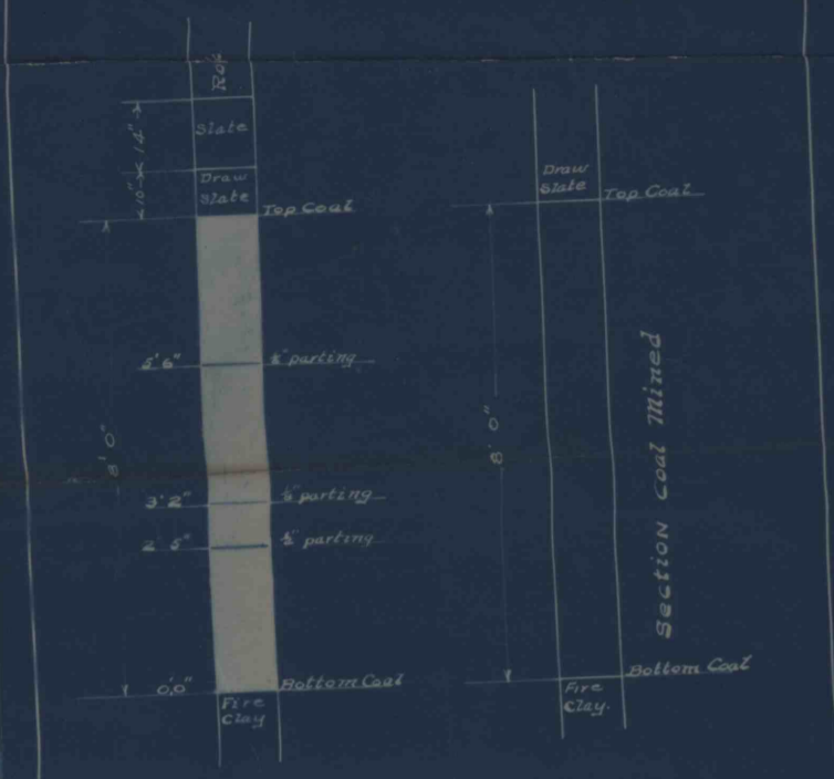
SECTION OF PITTSBURGH COAL VEIN UNION CONNELLSVILLE COKE CO. UNIONTOWN FAYETTE CO. PA. Scale 5" = 1' May 11-1920.
