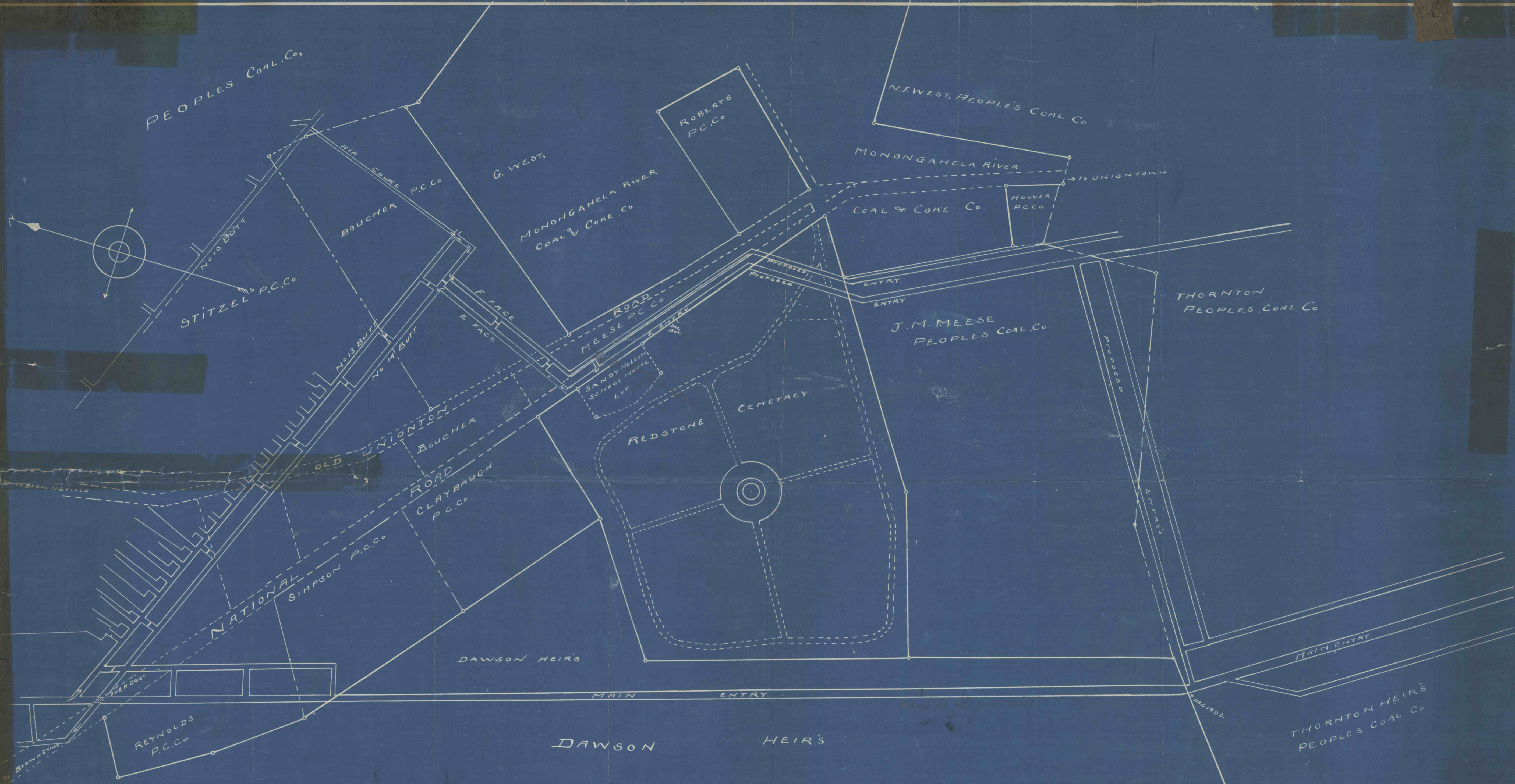
PLAN SHOWING LOCATION OF MAIN ENTRY AND AIR COURSE AROUND REDSTONE CEMETRY PIKE MINE PEOPLES COAL COMPANY BROWNVILLE PA, SCALE 1" = 100 FT. DEC 23 rd 1902
