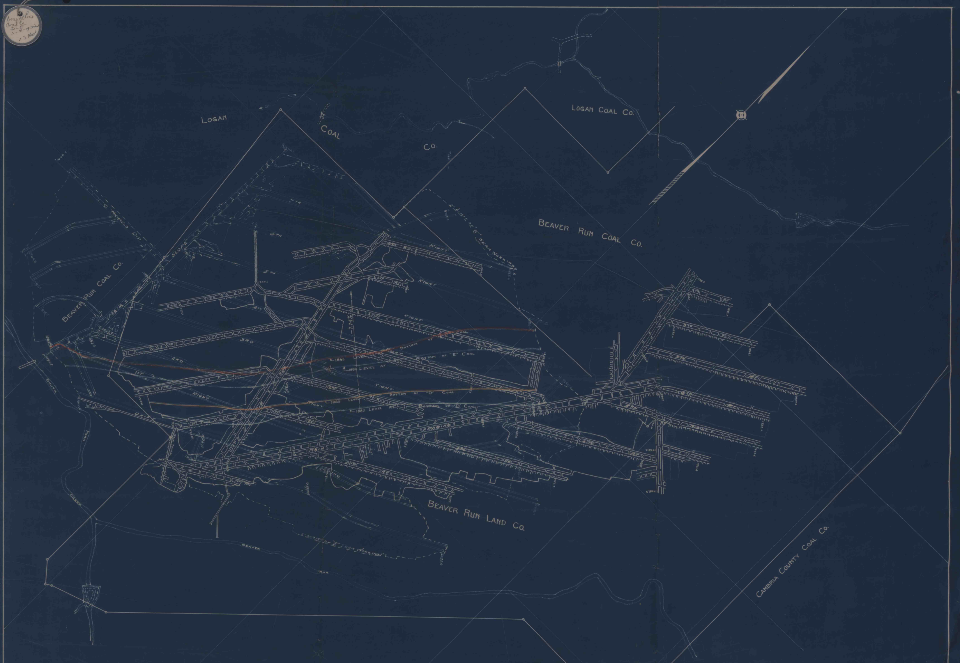
BEAVER RUN COAL CO. MAP SHOWING ELEVATIONS AND DRAINAGE IN "D" AND "E" SEAMS BEAVERDALE, PA. SCALE - 1" = 400' GRAY & CLAFLIN, ENGRS. JOHNSTOWN, PA. MAY 10, 1932.
