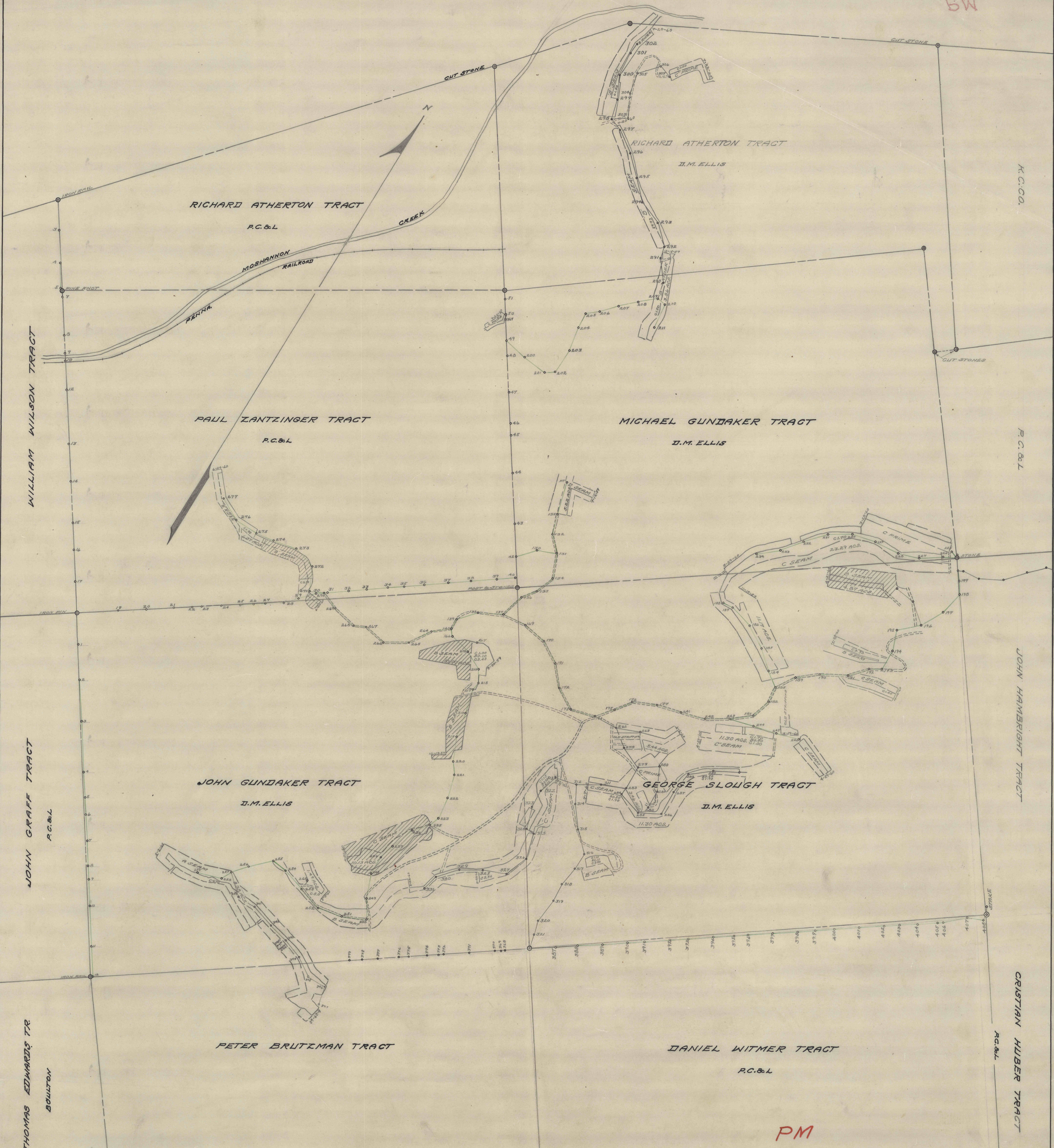
MAP SHOWING A, B, BRIDER, C, C' AND D STRIPPINGS OPERATIONS OF THE ELLIOT COAL MINING COMPANY ON THE I.M. ELLIS AND P.C. & L PROPERTIES IN RUSH TOWNSHIP CENTRE COUNTY PA. SCALE 1" = 400'
