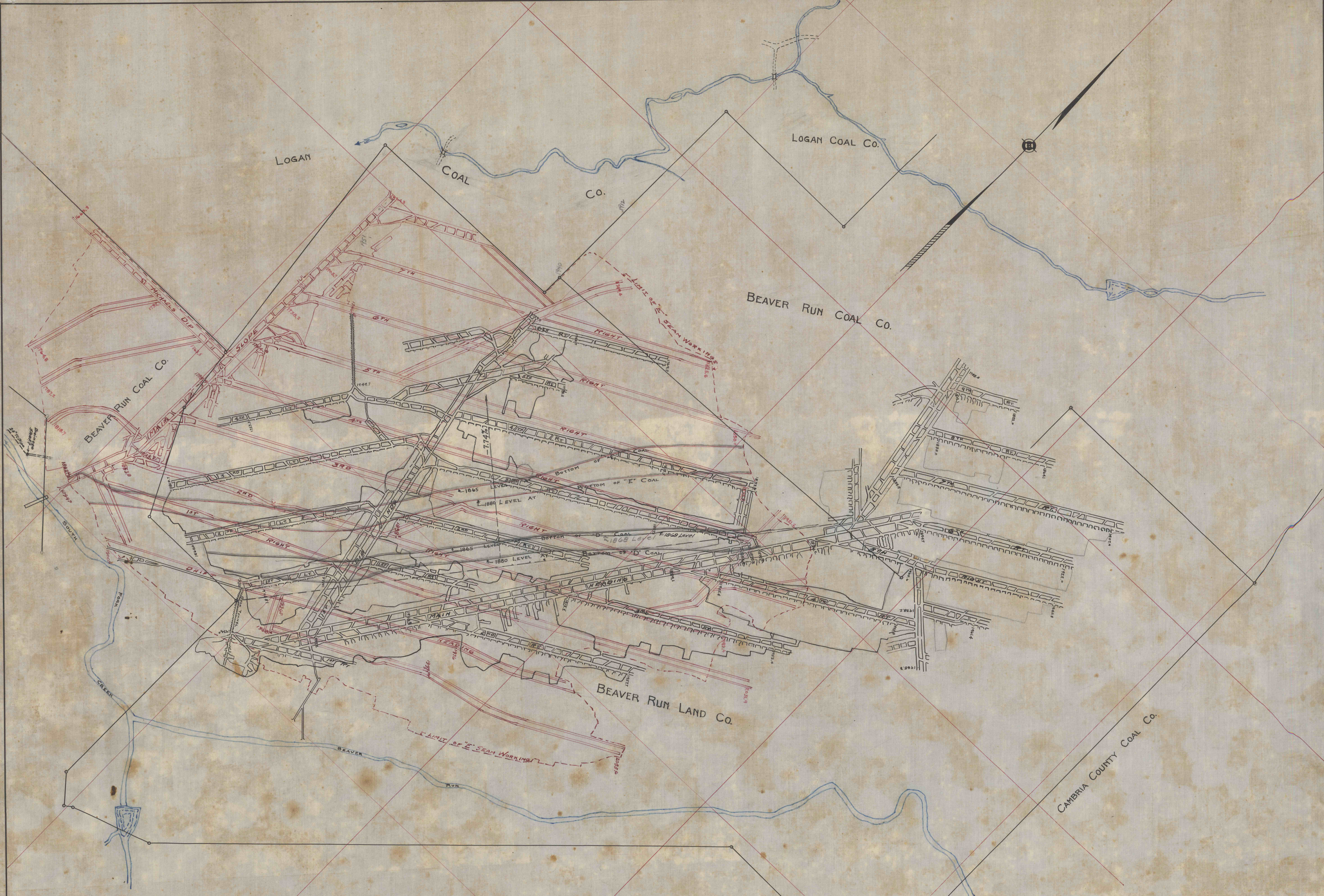
BEAVER RUN COAL CO. MAP SHOWING ELEVATIONS AND DRAINAGE IN "D" AND "E" SEAMS BEAVERDALE, PA. SCALE - 1"=400'
