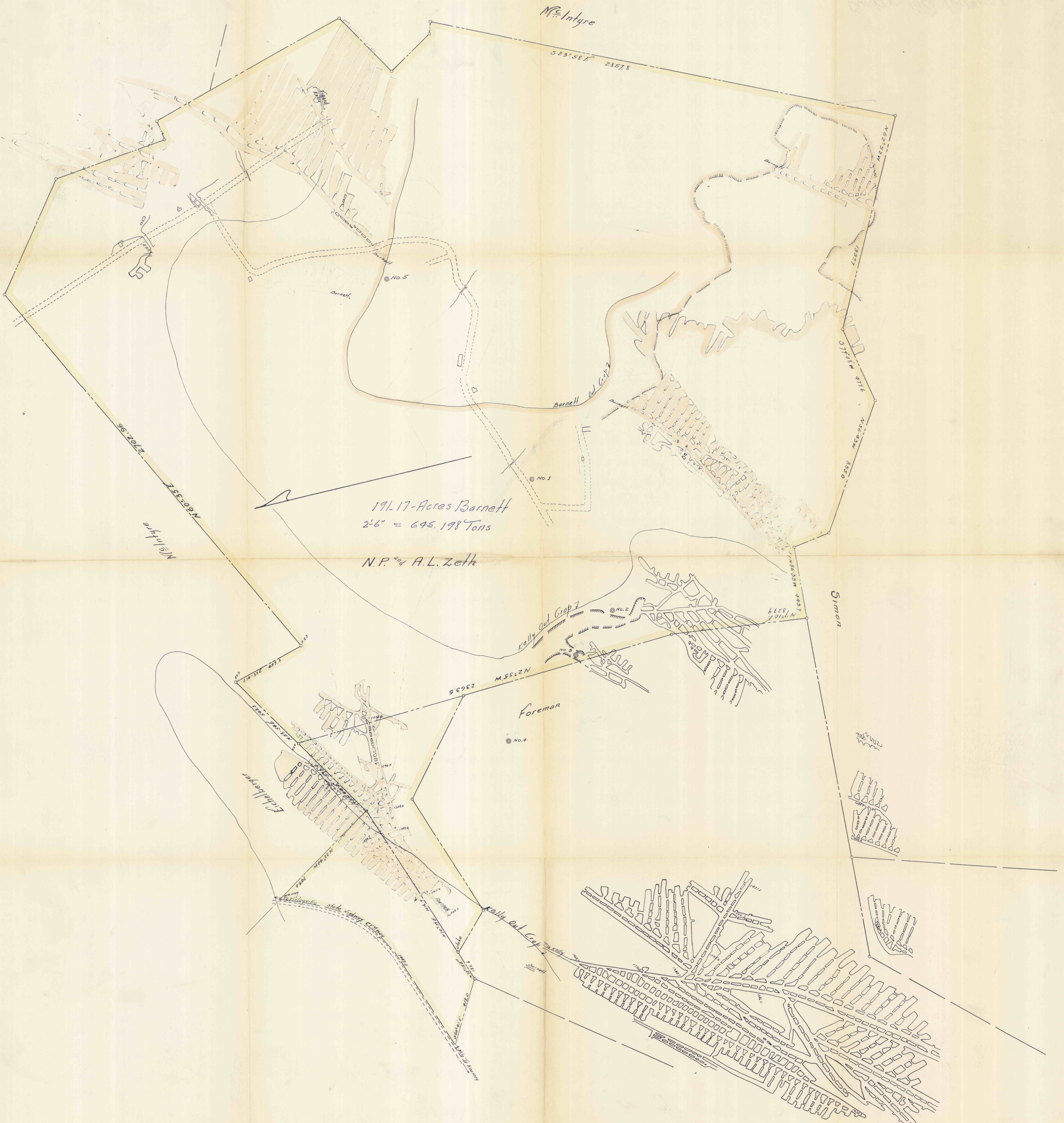
Map Showing Coal Remaining In N.P. Zeth Bunker Hill Property Situated In Broad Top Twp Bedford County Pennsylvania Barnett Seam May 1961 1" = 200' R. Carrio Eng. Robertsdale Pa.
