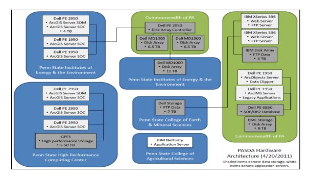
Figure 1. PASDA Hardware Architecture. Penn State HPC architecture is shown on lower left of diagram. This new hardware/systems allows a rearchitecting of existing PASDA resources.
